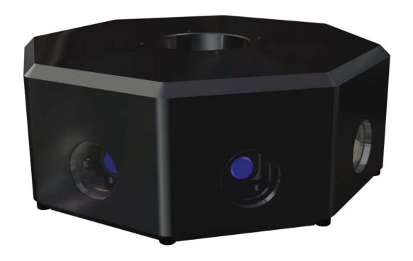
The Ring Camera provides a live 360 deg image, by stitching 8 full HD camera images together into a single HD-SDI output. Video stitching is carried out by a dedicated FPGA and requires no moving parts. Stand alone or integrated into a PTZ system the ring camera provides useful 360 deg local situational awareness for both military and policing activities.
